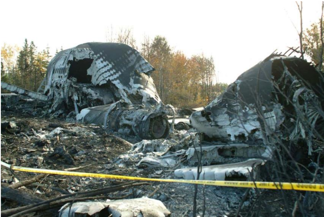
Figure 3 - The remains of the main fuselage and number 4 engine from MK Airlines flight 1602
